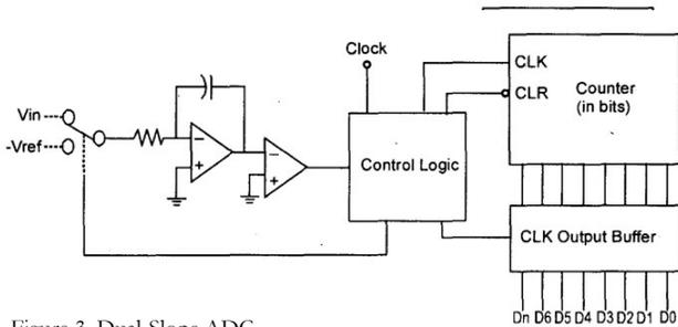
Figure 3. Dual-Slope ADC
