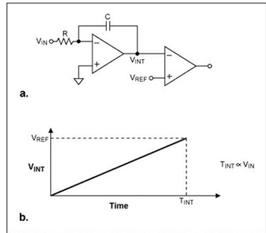
Figure 2. Single-Slope ADC.
